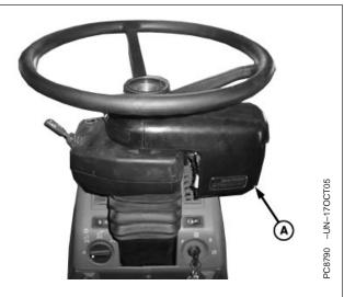
A-Steering Unit attached in 3 o'clock position
